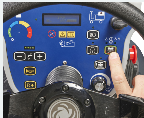
Brush deck/squeegee lowers automatically, minimizing operator effort
